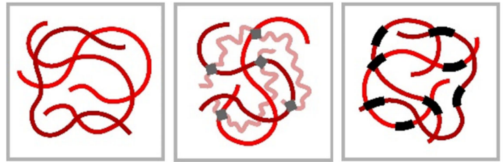
Figure 1 Vulcanization: Cross-linking elastomers to give unique properties
